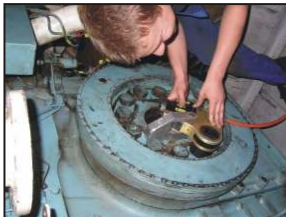
Service on diesel engines of ships with in-out socket and special reaction arm
